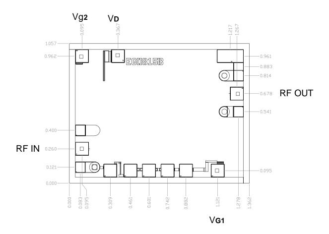
Units: millimeters Thickness: 0.1
