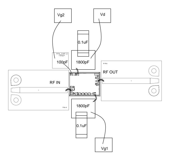
3 (Three) 0.7 mil chisel bond wires at RF IN and RF OUT or 1 (one) 3 mil ribbon at RF IN and RF OUT. Vg2 is optional for the circuit.
